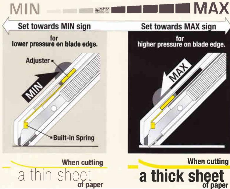
Hold the TS-1 as you hold a pen, and give it enough pressure to leave no space between the TS-1 and a sheet of paper while cutting.
